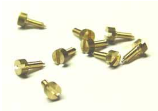
Fig. 11. Brass cheese head screws to hold the rotor movement together. Only three will be used, so servicing the next rotor will go much faster since the screws are already made.
