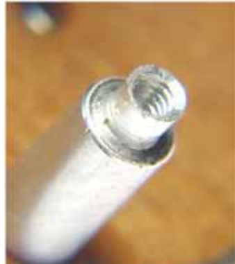
Fig. 10. The pillar posts must be drilled and tapped to hold a 0-80 screw so the plates can be put back together.
