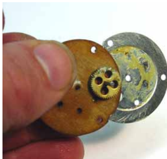
Fig. 9. The lubricant reservoir in the top plate, shown here, is easier to clean than the one in the bottom plate.
