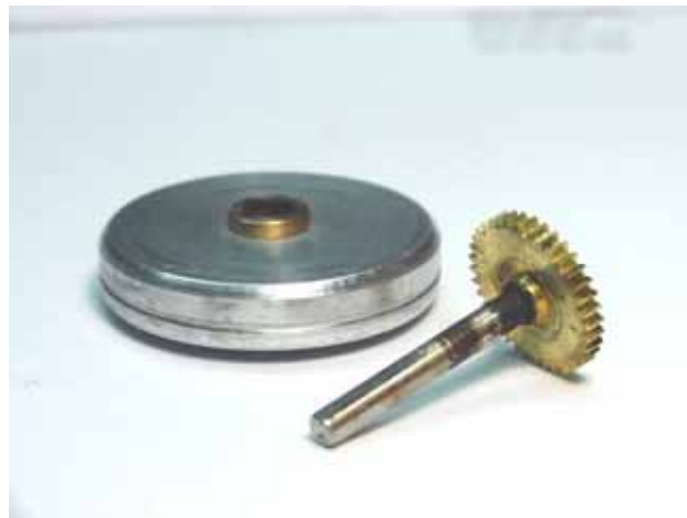
Fig. 7. The cap bushing and drive gear shaft are the two areas that need the most attention. Both require significant cleaning and polishing for the rotor to function properly.
