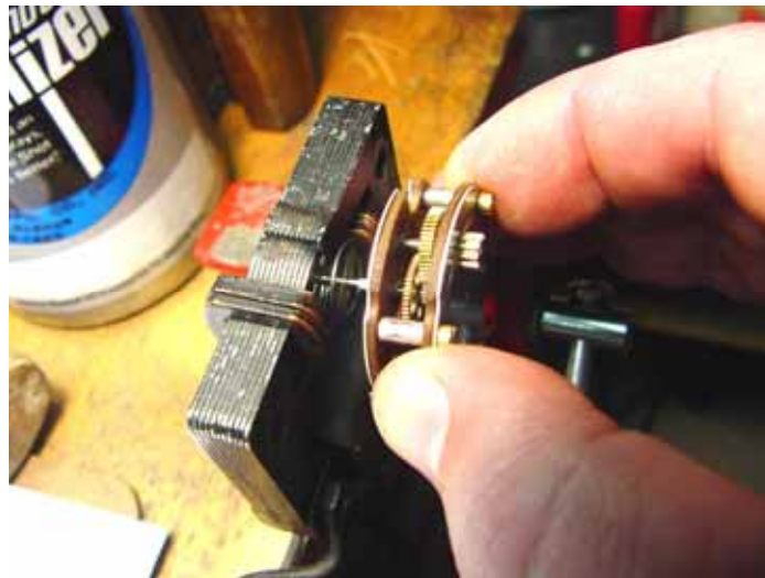
Fig. 15. The fun part! The freshly serviced movement can be tested by energizing the coil and inserting the armature in the magnetic field. Holding it just right allows the armature to spin within the field coil and an easy examination of the working movement.
