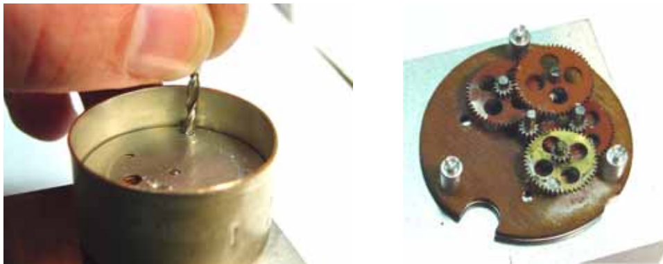
Fig. 5. To remove the top plate, the rivets on the posts must be removed. This operation must usually be done before the movement can be removed from the body of the can. Remove just enough material so the plate can be pulled off.
