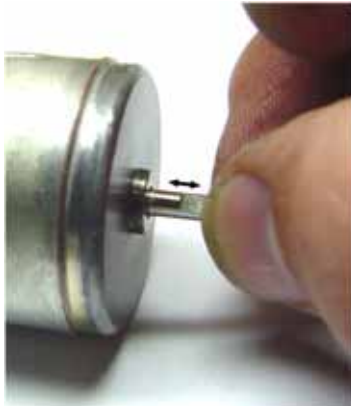
Fig. 17. Check the end-shake of the drive gear shaft. If there is none, the cap is on too tight.
