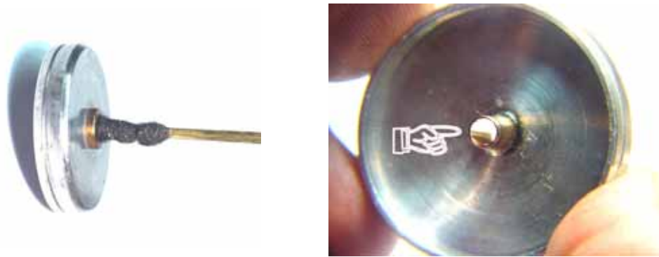
Fig. 8. Cleaning the cap bushing. Steel wool on a toothpick is useful for cleaning out the old, dry oil.
